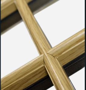
In order to meet modern building regulations and because we are not constrained by glass technology of the period, Residence 9 is made from complete pieces of glass where glazing bars are clad to the glass rather than making individual, small glass units. Internal spacer bars give the appearance of individual units, with the performance of a single, larger sealed unit.
